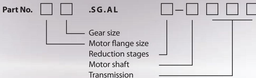
Planet gears **SG.AL** AL with hardened, integrated gearing, high strength and precision at minimum dimensions offer furthermore:
